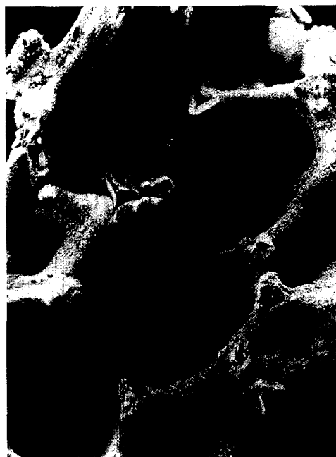
Fig. 2. Scanning electron microscope picture ( \times 100 ) obtained for \text{PbO}_2 deposited on RVC from a nitrate solution.
